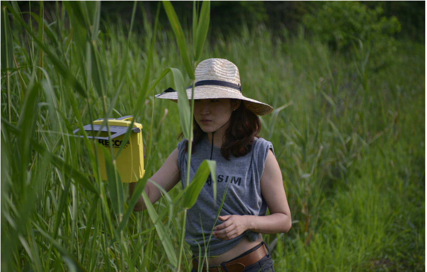
Fig. 3: We used harmonic direction finding, which relied on a microwave emitter and light-weight reflectors, to study the diel cycles of microhabitat use during the breeding season in two treefrog species. The student in the picture tried to locate an individual treefrog by listening to the pinging sound uttered when a microwave reflected from the reflector that was belted on the treefrog was returned to the emitter.
